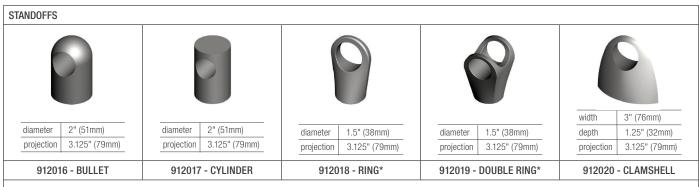
\*Series 1200 Ring and Double Ring standoffs are slightly different in design compared to their Series 800 counterparts. Series 1200 standoffs return to the mounting surface with a round cross-section. Series 800 standoffs return to the mounting surface with a rectangular cross-section.
